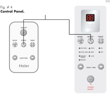
Timer On or Timer Off mode is used to pre-start or shut off your unit in advance. You can program this up to 24 hours in advance. You can use the Timer in 4 functions, i.e. COOL, ENERGY SAVER, DEHUMID or FAN.
